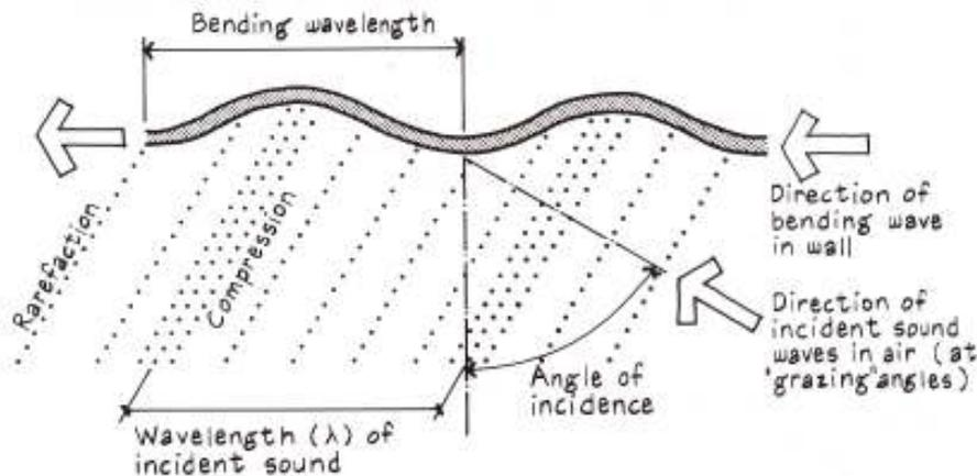
To achieve high TL performance, use double-wall constructions with wide separation between layers, **light-gauge metal studs instead of wood studs**, or metal channels to "resiliently" support gypsum board layers. These elements, if properly installed, can **reduce the stiffness of a barrier. The ideal sound-isolating construction would be heavy, limp, and airtight!** (Acoustiblok is "heavy, flexible, and airtight"!)
