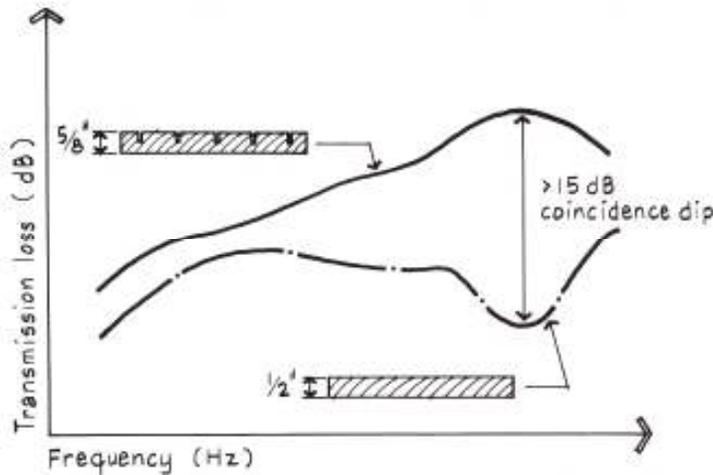
As shown by the above graph, the coincidence dip can be greater than 15 dB for stiff materials. **This significant difference in TL is caused by the altered response to bending waves, which are excited by the impinging sound energy.** Bending waves are similar to the wave motion in a rope shaken at one end. The exaggerated sketch below shows bending-wave coincidence for a wall.
